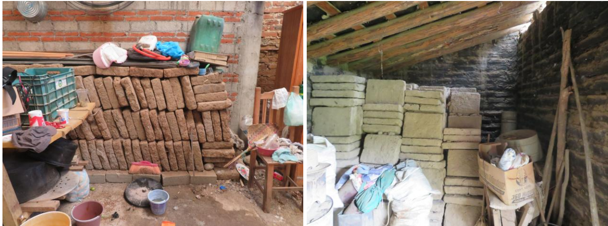
Figure 6 & 7: Century-old adobe bricks are carefully set-aside and reserved for future use in Santo Domingo Tomaltepec. (Source: Catherine Sckerl, 2025).
