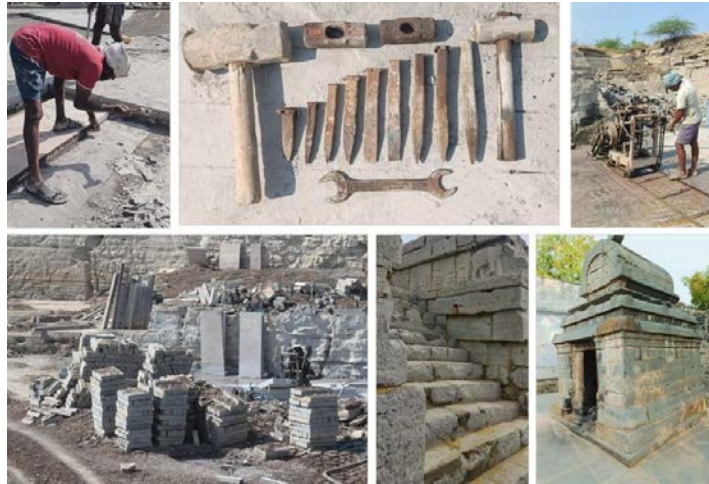
Figure 3: Extraction practices using machines as well as hand tools, stone modules, historic examples of kadapa stone construction. (Source: Authors).
