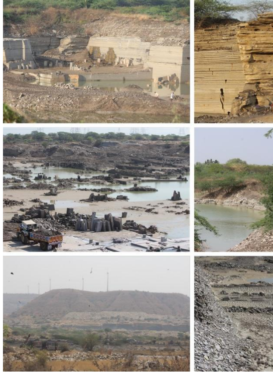
Figure 2: Geological formations of kadapa stone such as outcrops and subsurface quarry, stratification, expanse, extant quarry. (Source: Authors).
