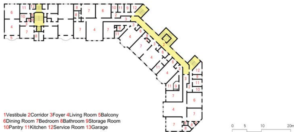
Figure 10: Typical floor plan of the Brookside Apartments (Source: Drawn by the author).
