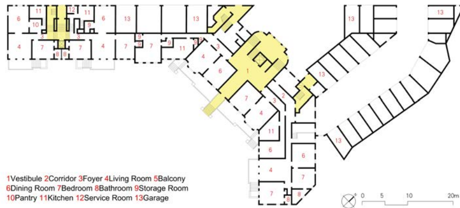
Figure 9: Ground floor plan of the Brookside Apartments (Source: Drawn by the author).
