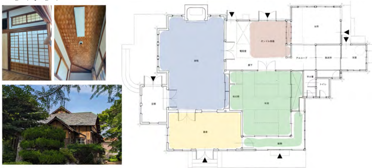
Figure 6. In the reconstruction map 32 , blue is the reception room, yellow is the study, green is the tatami room, and red is the Ondol room. Traditional Japanese techniques can be seen from the Yukimi shoji window 33 (top left) and the Ajiro ceiling 34 (top right.)
