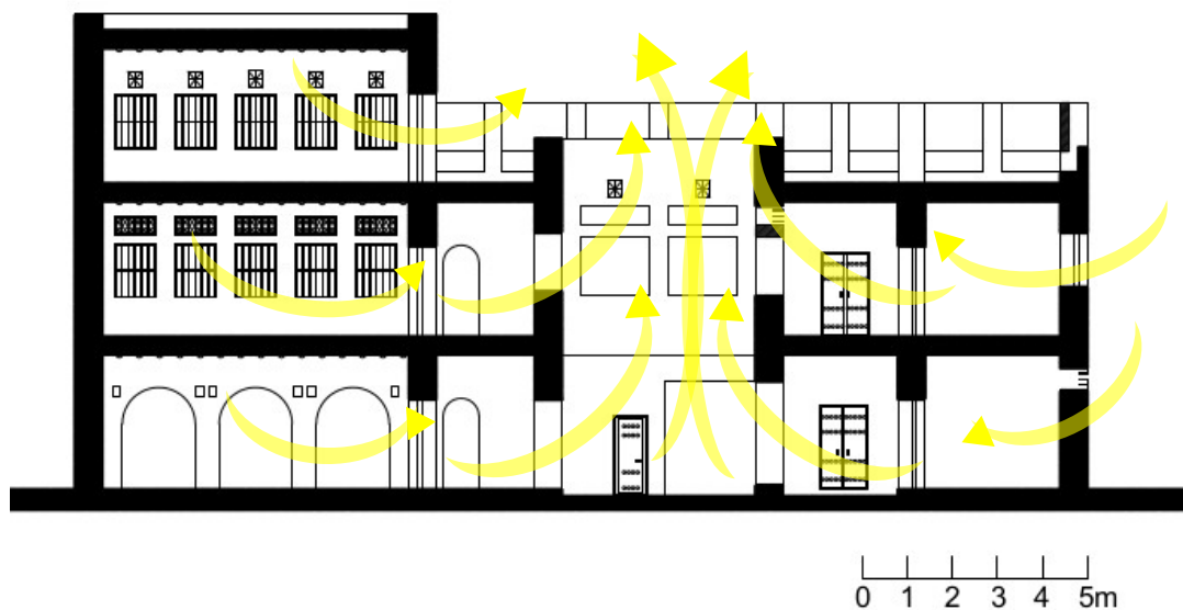
Fig. 11: The stack ventilation effect created by the courtyard form and the openings. (Source: By the author)
