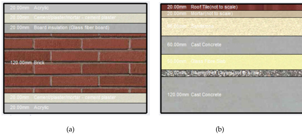
Fig.8: The thermal properties of the insulation tested materials (a) walls & (b)roofs. (Source: The researcher).
