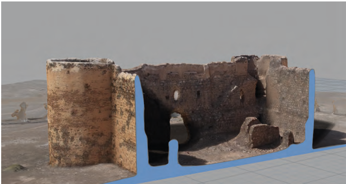
Fig 24: The Extraction of plan and sections reveal the internal details and structure of the building (Author, 2023)
