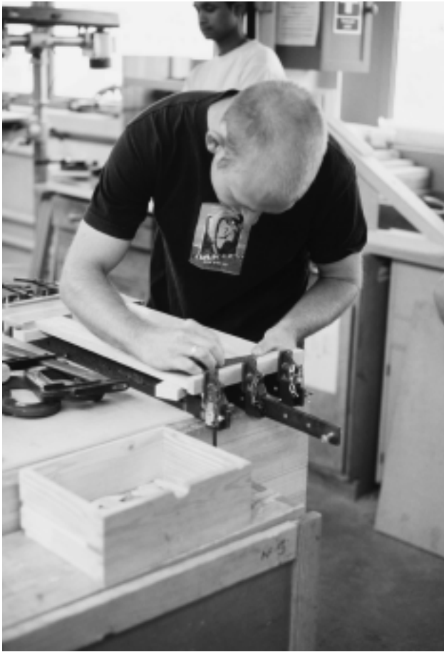
FIGURE 9. Woodworking student, Toby, cramping a component for a piece of furniture at the workbench.
