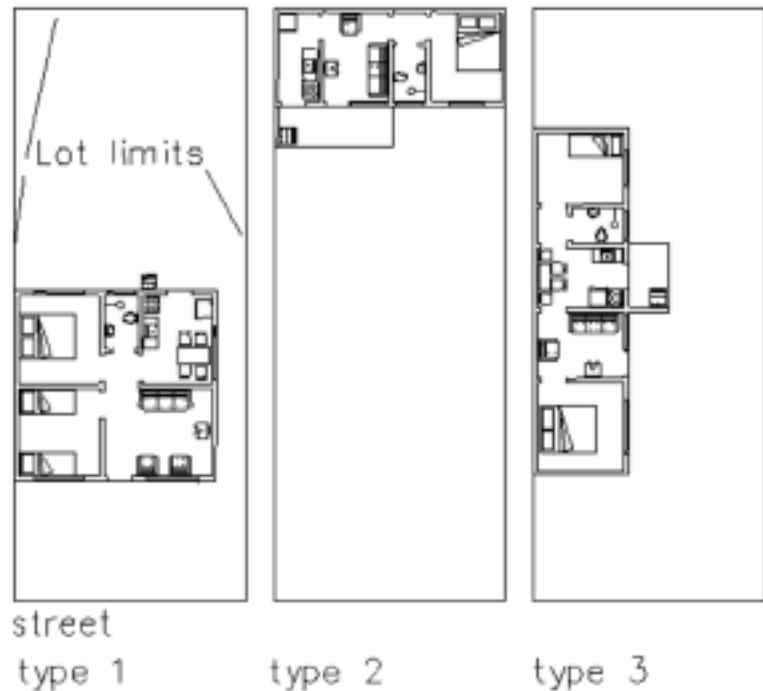
FIGURE 5. Schematic site plans and elevations of pre-dominant types of self-built houses in the Campinas region.
