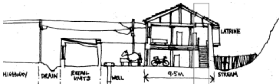
FIGURE 7. Section through a tourist hostel in an existing Tibetan building next to the main street in the town of Thlagong. The box on the right indicates the main (physical and spiritual) vertical organization. (Drawing by Nic Crawley, 2000.)
