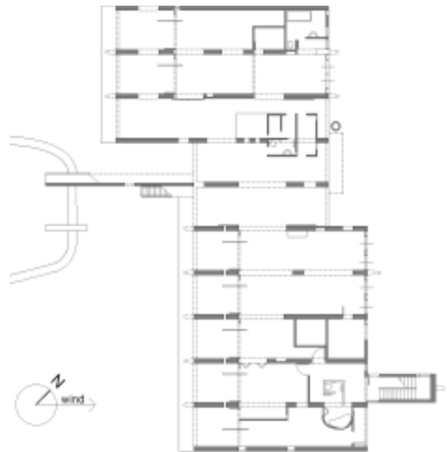
FIGURE 20. Detail of first floor plan of the house opened up for the night.
