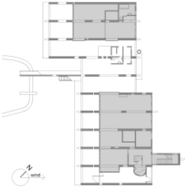
FIGURE 13. Detail of first floor plan, showing house closed for the summer afternoon.
