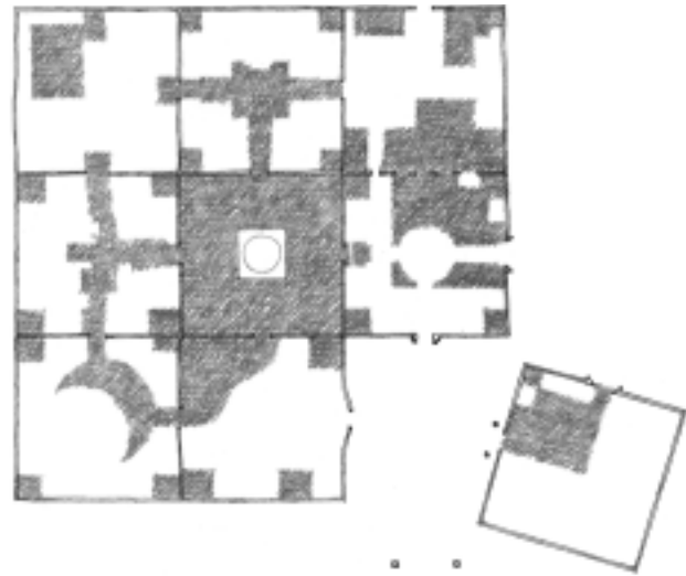
FIGURE 10. Plan of Jawahar Kala Kendra, showing the “misplacement” of one of nine squares in the mandala. (Courtesy of the office of Charles Correa, architect, Bombay.)
